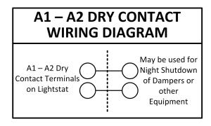
Use #18 gauge 2-conductor twisted pair cable between the Lightstat **TME** and the damper or equipment to be shut down.
