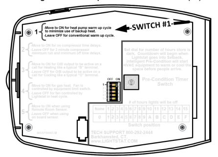
**Note**: The Lightstat **TME** must be powered Off and On in order to "read" a change of switch settings. Moving this switch to the ON position will increase the heating Setback by  $5^{\circ}$  (F). This will allow a heat pump to stay in a compressor mode longer and avoid expensive electric resistance heat.
