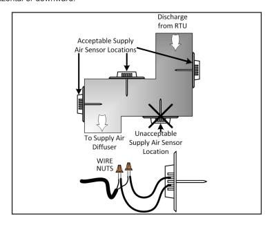
Use #18 gauge 2-conductor twisted pair cable between the Lightstat **TME** and the Supply Air Sensor. Supply Air Sensor is unaffected by wire runs of up to 500 feet.
