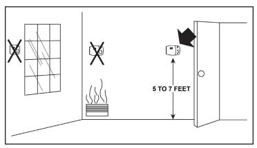
Pick a mounting location **AWAY** from drafts, windows, doors, outside walls, and heat vents. Relocate if necessary.
