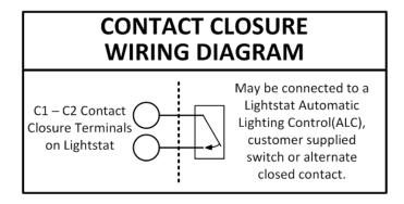
Use #18 gauge 2-conductor twisted pair cable between the Lightstat **TME** and the customer supplied switch or alternate closed contact.
