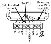
**Note**: When connecting a Lightstat TME to a heat pump with **Thermostat Reversing Valve Control** you will need to install a jumper wire between W1 and Y1 at the Lightstat TME as shown in the diagram above.
