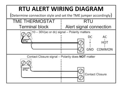
The Lightstat **TME** has a visual alarm to indicate that there is a problem with the Roof Top Unit (RTU). This is a field option. You might not have this option with your specific RTU.
