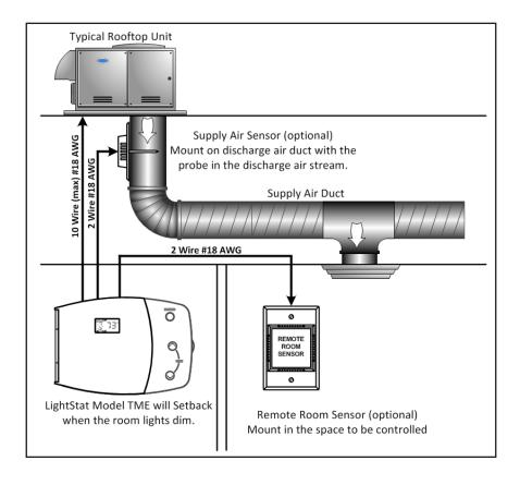
**Note:** All wiring should be minimum #18 AWG. Shielding is **not** required.
