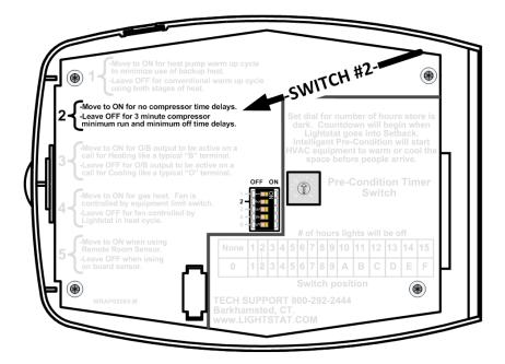
**Note**: The Lightstat **TME** must be powered Off and On in order to "read" a change of switch settings.
