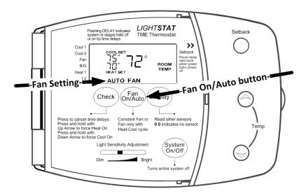
The **CHECK** button is used to cancel any safety time delays. These time delays are to protect the equipment from short cycling, and to prevent multiple HVAC systems from coming on at the same time after a power failure or with the lights. If you see the word **DELAY** flashing, then the Lightstat **TME** is in a time delay. The startup time delay can be as long as 12 minutes.
