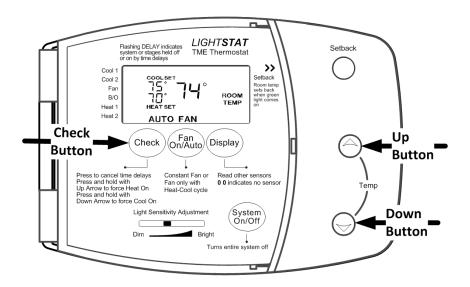
You can also force the **Cooling** on by pushing the **Down Button** and the **CHECK** button at the same time. This will force the cooling on while you are pressing both buttons.
