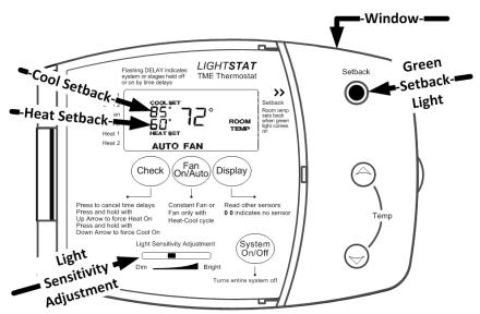
NOTE: The light adjustment slide is recessed in the slot.
