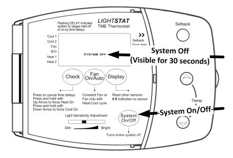
Use the **DISPLAY** button to shift the temperature display from **ROOM** temperature to **SUPPLY** temperature. The **SUPPLY** temperature is the air temperature coming from your HVAC system. You will have to install a Supply Air Sensor in order to read this temperature. If you do not have this sensor installed, then the display will read "**00**".
