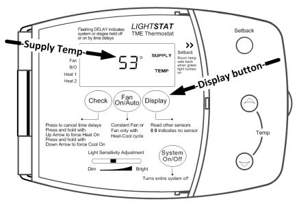
The **FAN ON/AUTO** button will shift the fan operation from continuous to cycling with a call for heating or cooling. If the fan is left in the **FAN ON** mode during occupancy, it will automatically shift to **AUTO FAN** during Setback.
