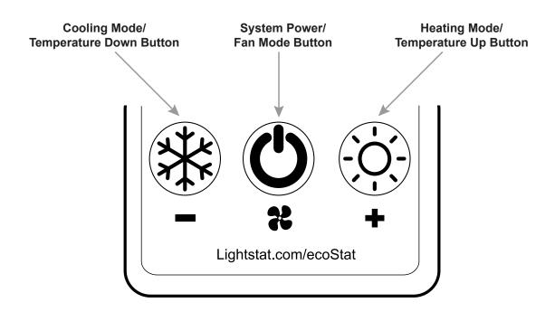
Each button has a **long press** function (more than 2 seconds) and a **short press** function (less than 2 seconds). The following tables show the typical function of each button:
